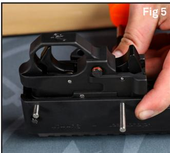
5 It is not recommended to disassemble the trigger guard any further. The inside of the trigger guard should be cleaned periodically. When cleaning the trigger guard, use an aerosol gun cleaner that leaves no residue. **DO NOT** spray any oil onto the hammer/sear engagement area. Be sure to remove any excess over spray with a cotton swab.
