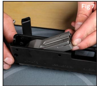
**8 DO NOT** disassemble the bolt any further. The inside of the receiver should be cleaned and minimally lubricated on a regular basis using any quality gun oil.
